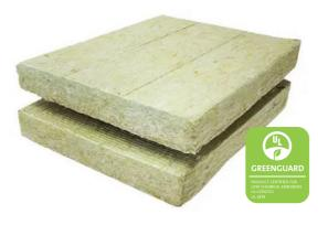
JM CladStone<sup>™</sup> 45 Insulation is made of inorganic fibers derived from basalt, a volcanic rock. Advanced manufacturing technology ensures consistent product quality, with high-fiber density and low shot content for excellent performance. JM CladStone 45 is inorganic, noncombustible, moisture repellent, non-deteriorating, and will not mildew or support corrosion.
